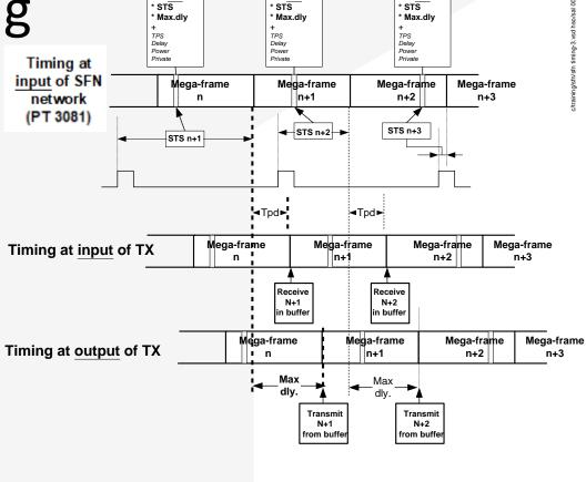
Transmit time (STS clock) = STS + Max delay +/- Loc.dely +/- Opt.delay
